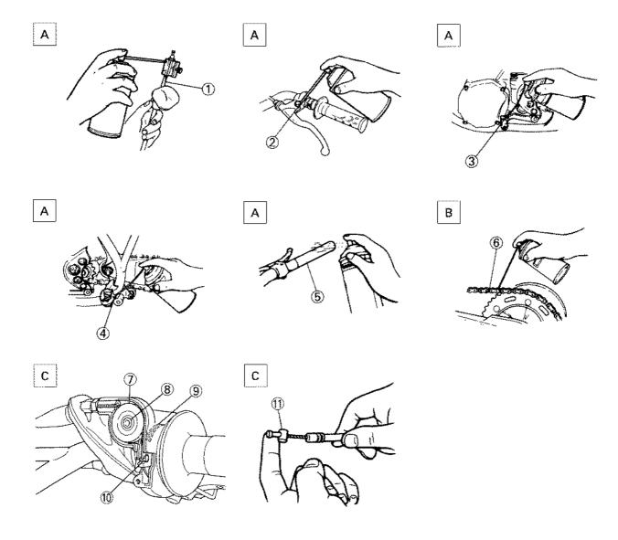
To ensure smooth operation of all components, lubricate your machine during setup, after break-in, and after every race.
