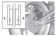
1. Brake pad wear indicator groove
