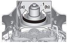
1. Spring preload adjusting bolt
