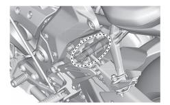
The pivoting points of the rear suspension must be lubricated by a Yamaha dealer at the intervals specified in the periodic maintenance and lubrication chart.
