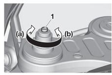
Compression damping force adjusting screw
