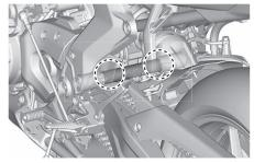
The swingarm pivots must be lubricated by a Yamaha dealer at the intervals specified in the periodic maintenance and lubrication chart.
