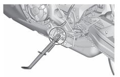
The operation of the sidestand should be checked before each ride, and the sidestand pivot and metal-to-metal contact surfaces should be lubricated if necessary.
