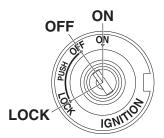
The main switch/steering lock controls the ignition and lighting systems, and is used to lock the steering. The various positions are described below.
